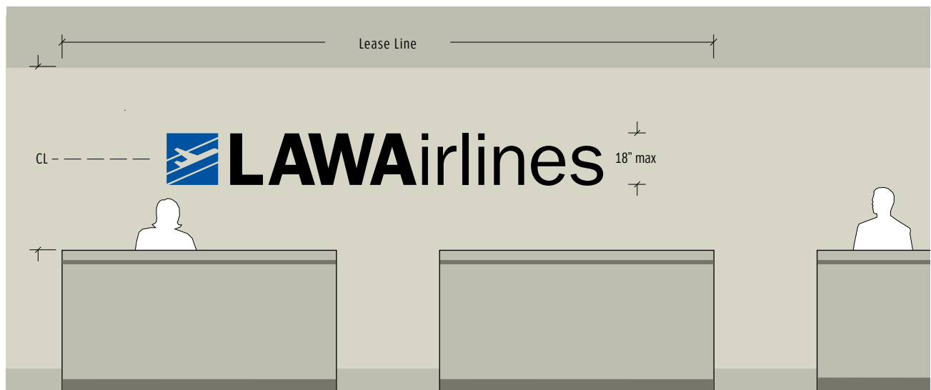
Figure 3c: Dimensional copy is the preferred treatment for corporate signature signs on walls behind ticket counters.
