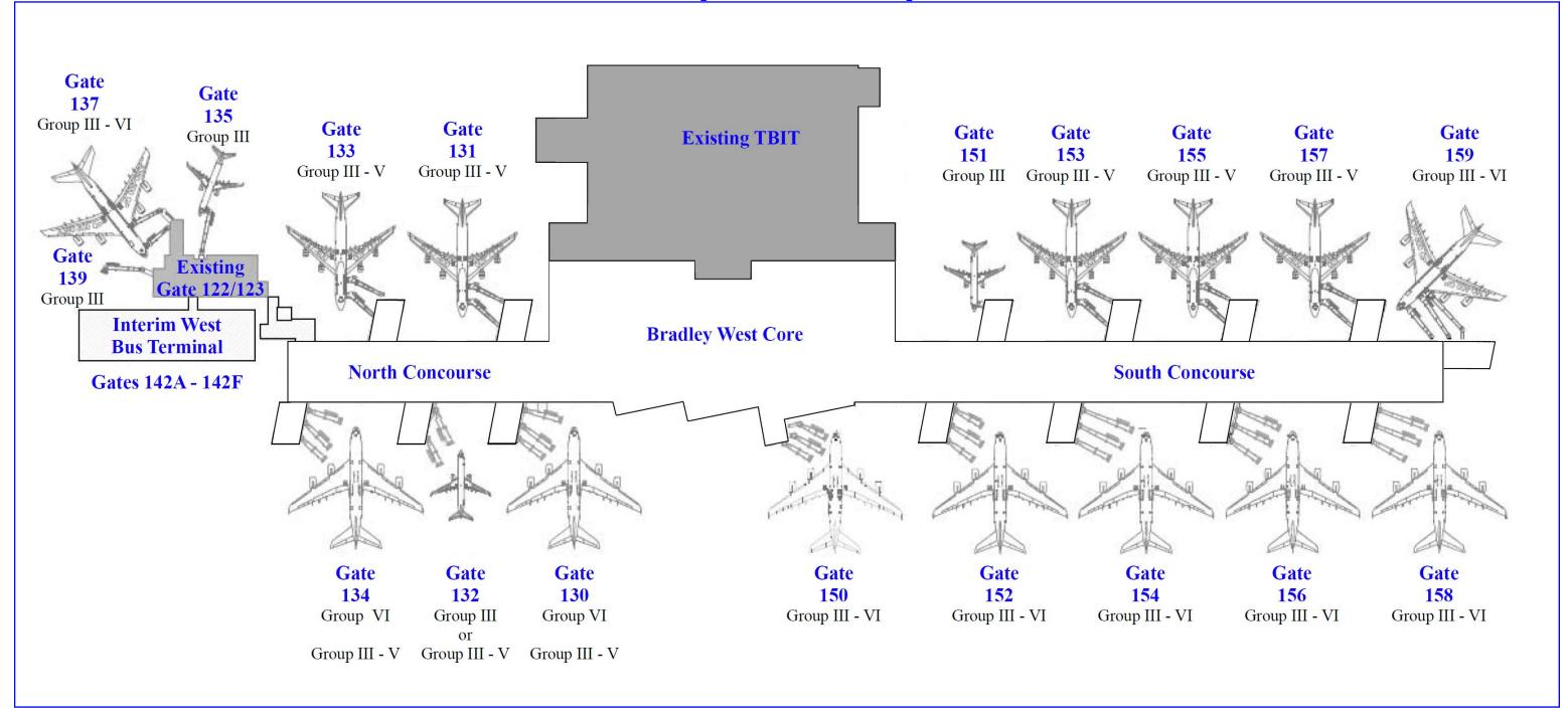
To supplement the article in this newsletter about the increase in A-380 service to TBIT, the above drawing shows the aircraft parking layout and Aircraft Design Group (ADG) that each gate can accommodate upon completion of the Bradley West Program. The west side of the concourse as well as the north and south ends (with the exception of Gate 132) are designed to accom-
