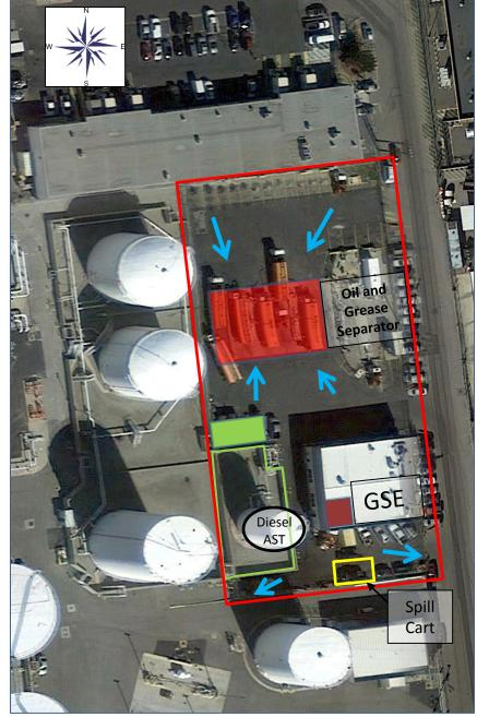
Note 1: Diesel AST is contained with 6" berm
