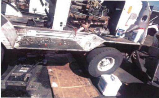
Photo 17: Poor housekeeping and poor management practices were observed here. Oily equipment was observed stored outdoors without containment or cover. Oil spills were observed on the ground.
